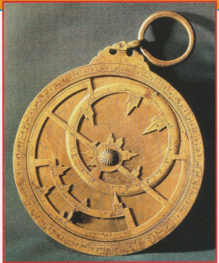
A 9th-century astrolabe. Astrolabes were used by early astronomers to calculate the position of the stars and planets. They were also used as navigational devices.
